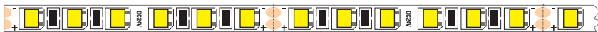
High luminosity flexible led strip, 24V, IP20, 5mm PCB. It can be cut every 8 leds.
