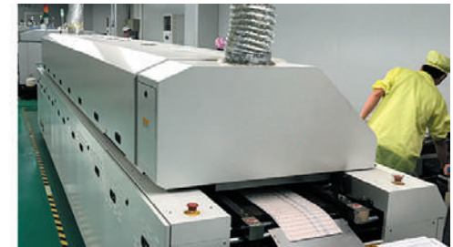
Drying oven for sealing soldered parts
