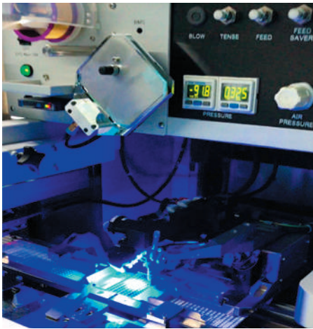
Machine soldering with gold wires
