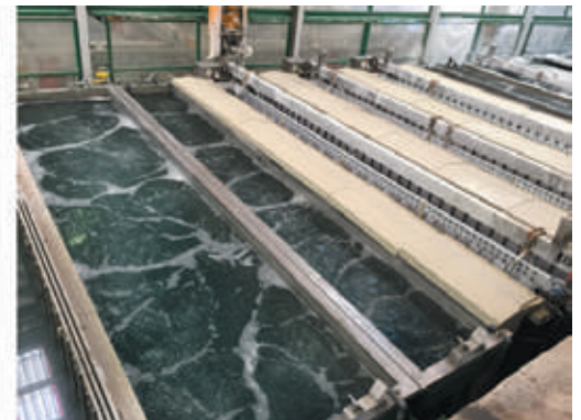
Profile anodising process
