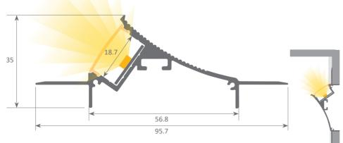
Aluminum led profile + cover designed to offer indirect and soft linear lighting. It is finished off with a layer of plaster making it completely integrated in the wall. It can be used on walls or ceilings.
