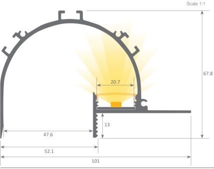
Aluminium led profile + cover intended for illuminating ceiling perimeters in rooms, giving diffused and ambience lighting. It is finished off with a layer of plaster making it completely integrated in the wall.
