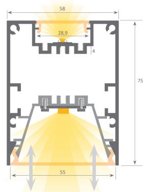
System with front removable tray which permits easy access to the led strip and power supply, therefore allowing very fast and simple maintenance of the electrical installation.
