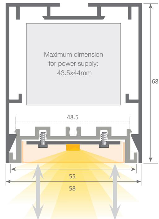
System with front removable tray which permits easy access to the led strip and power supply, therefore allowing very fast and simple maintenance of the electrical installation.
