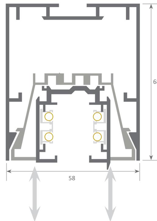
System with front removable tray which permits easy access to the led strip and power supply, therefore allowing very fast and simple maintenance of the electrical installation.
