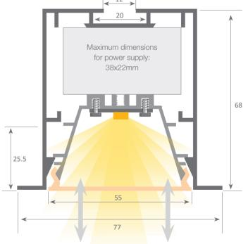
System with front removable tray which permits easy access to the led strip and power supply, therefore allowing very fast and simple maintenance of the electrical installation.
