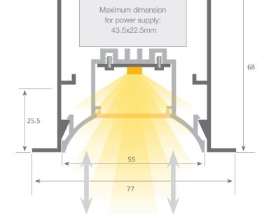
System with front removable tray which permits easy access to the led strip and power supply, therefore allowing very fast and simple maintenance of the electrical installation.
