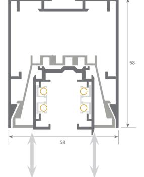
System with front removable tray which permits easy access to the led strip and power supply, therefore allowing very fast and simple maintenance of the electrical installation.
