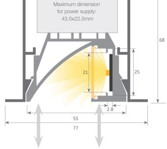
System with front removable tray which permits easy access to the led strip and power supply, therefore allowing very fast and simple maintenance of the electrical installation.
