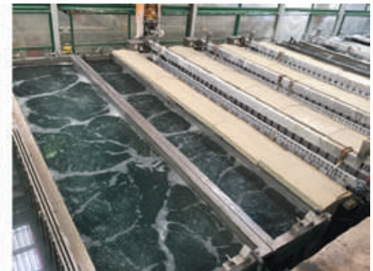
Profile anodising process
