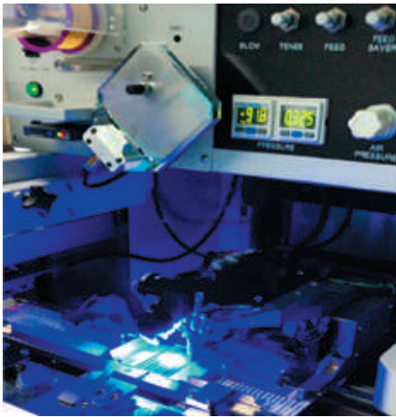
Machine soldering with gold wires
