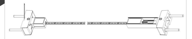
Soft Line is a new concept in linear luminaires and offers indirect wall and ceiling lighting. It consists of two supports that are fixed to the walls, ceilings or floors and both are joined by a thin steel plate where we will attach the led strip that we want to use. The steel plate measures 30 metres and we can cut it, meaning we can adjust the size of our luminaire.
