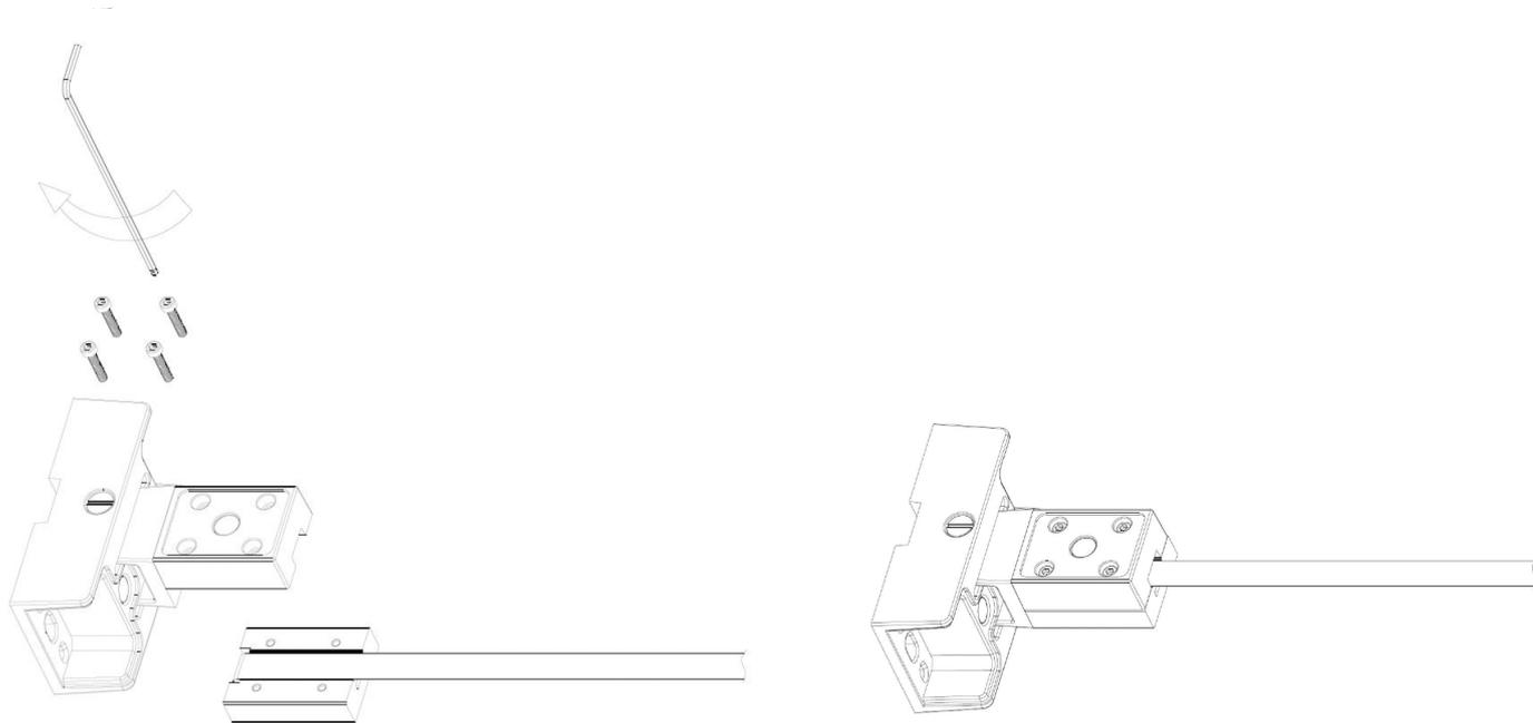
2. Installing the steel plate onto the long support
