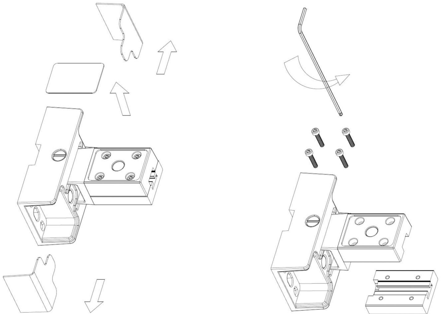
First, we will remove the external trim caps, access the interior and remove the 4 hexagonal head screws
