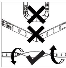
part. Never bend to an angle of 90°. It can have a radius of ≥20mm or an angle of 180°.
