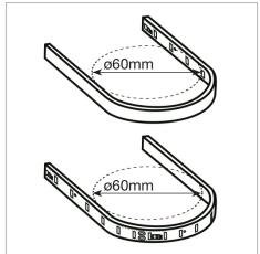
4. The bending diameter of the flexible strips must 5. Flexible strips cannot be bent by the welding 6. Fix by removing the back tape protector. not be more than ø60mm.
