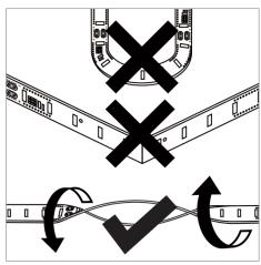
part. Never bend to an angle of 90°. It can have a radius of ≥20mm or an angle of 180°.
