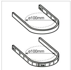
4. The bending diameter of the flexible strips must 5. Flexible strips cannot be bent by the welding 6. Fix by removing the back tape protector. not be more than ø100mm.
