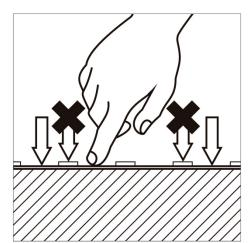
7. When applying the strip, press between the 8. The use of an aluminium profile is recommended 9. Only handle the flexible strip when off unwind leds and not on the surface of the led.
