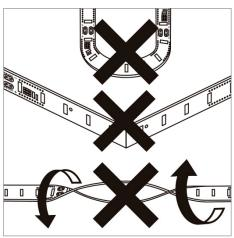
4. The bending diameter of the flexible strips must 5. Flexible strips must not be twisted or bent at 6. Fix by removing the back tape protector. sharp angles.
