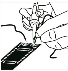
3. Polarity (+/-) must be respected. The soldering temperature must not exceed 360°.
