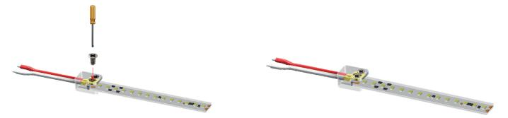
5. Once the screws are well fixed to the connector, we will cover it with the electric feed end cap. Once it is in place, we will fill the endcap with transparent silicone ref: 22.140 to completely seal it.
