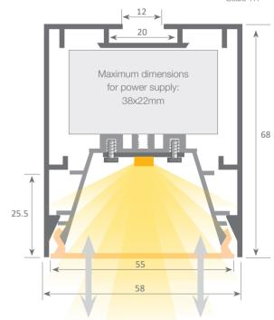
System with front removable tray which permits easy access to the led strip and power supply, therefore allowing very fast and simple maintenance of the electrical installation.
