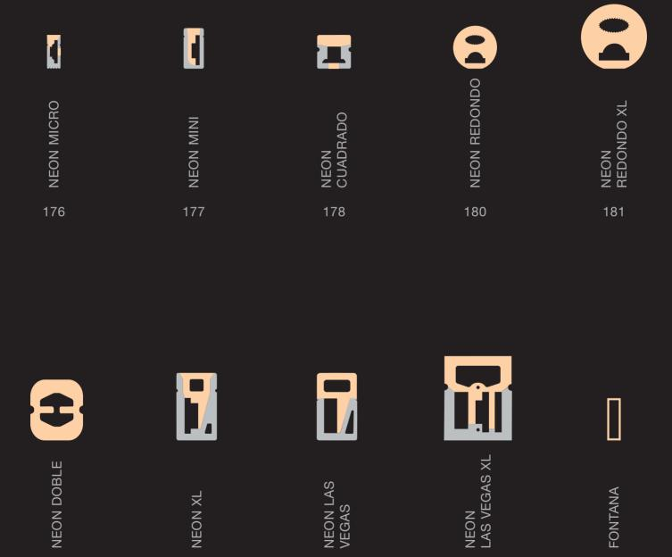
A very small, high quality silicone profile with an opal front. It is suitable for perimetral decorative lighting, illuminating cavities, etc. As it is extremely thin, it is also ideal for publicity texts and corporate letters on a small scale (its flexibility allows us to create very small letters).
