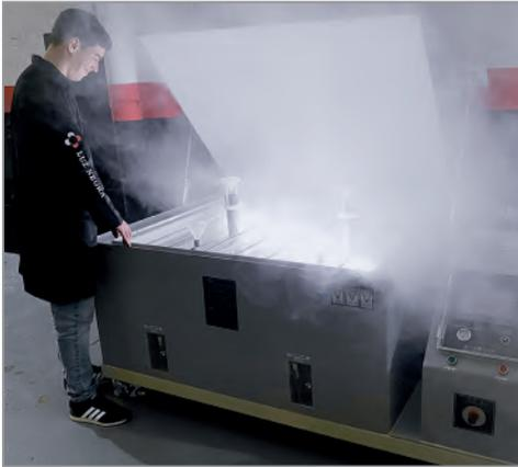
**Salt spray chamber (corrosion tester):**
