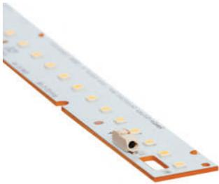
Constant current led modules for elevated luminosity and high performance linear luminaires. Designed in Germany and manufactured in the European Union, they have a 5-year warranty and a performance of up to 190 lumens/W. They can be fed from 150mA to 700mA and their measurements correspond to the Zaga standards of 140-280-560-1120mm (depending on the model). We have two models; premium that offers maximum luminosity and the ECO version that offers a highly competitive price.
