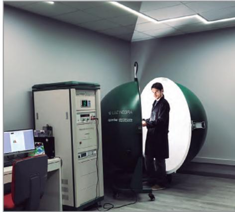
**Spectroradiometer with a 120cm sphere:**
